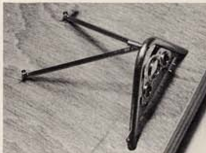
Figs. 5, 6, and 7. Three typical soldering jigs. (Above left) Using masking tape to hold four wire parts in alignment, and (below and below left) more-elaborate fixtures for soldering an auto dashboard and a complicated suspension part.
