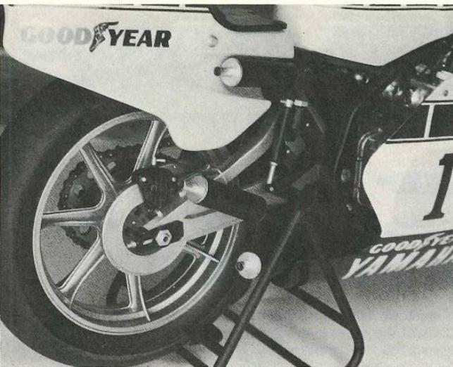
**Fig. 3.** Paul used the lathe to clean up many of the kit parts on this 1/12 scale motorcycle, including the mufflers and brake disc. The mounting studs for the fairing and the brake line connections were turned from brass.
