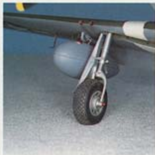
20. Here's the finished strut and wheel; each strut was machined from brass rod. Note the drop tank plumbing made from solder and wire.
