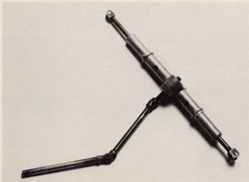
Fig. 13. Paul says that the universal joints in this 1/12 scale brass and aluminum steering assembly work perfectly, with no slop or binding.
