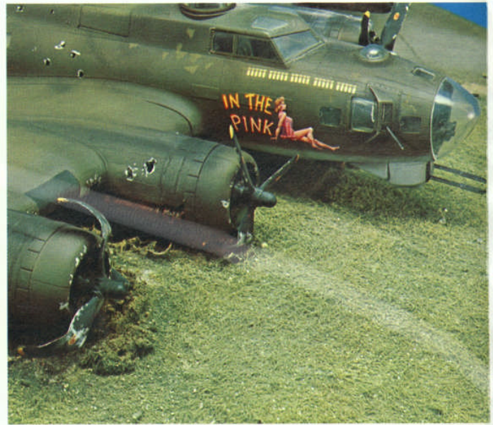
In that most B-17's taxied on their outboard engines, only the bottom blade of the inboard prop was bent, whereas the whirling blades of the outboard propeller were severely distorted by the mishap. The blades are bent as described in the text. Note the nose art on this B-17. Though you may wish to copy an actual aircraft, you can also create your own nose art, as our modeler did.
